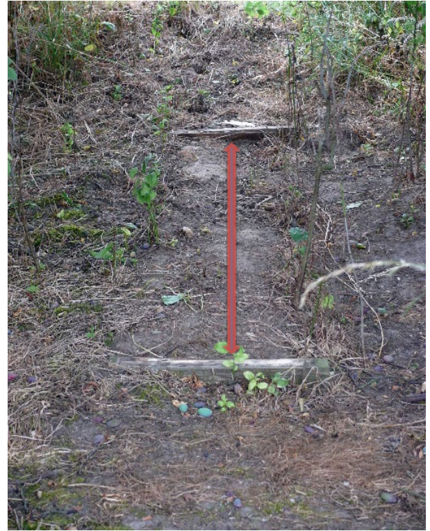
Two logs of wood (length ca. 30 cm) to put the trap in a small distance to the soil, for minimizing influence of water and extend life time of the trap
