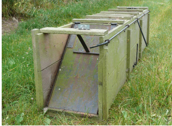
Trapping system triggered by a rocker board in the centre of the ground plate
