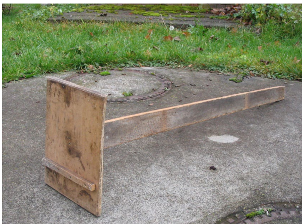
Instrument to push trapped animal into wire box (measurements according inside space of box trap)
